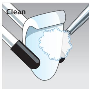
Clean with ultrasonic cleaner (e.g. 1 min, ethanol 70%) or steam cleaner (e.g. 5 s per unit, 4.5 bar).
