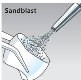
Sandblast the surface to be bonded with 25-50 µm aluminium oxide at 1.5 bar. **Note:** Do not etch the restoration with hydrofluoric acid.
